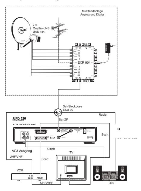
The DiSEqC switching matrix EXR 904 allows the connection of 4 subscribers.
